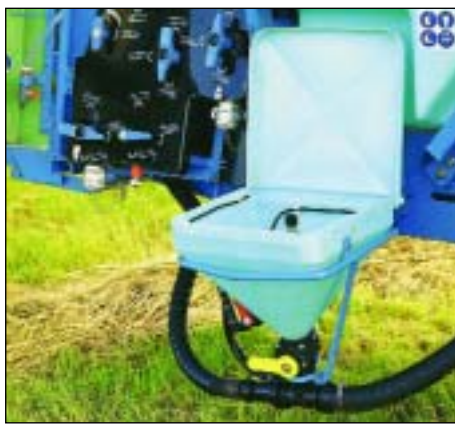
1 - Retractable chemical hopper, which is at man height at the time it is used and does not damage the vegetation during spraying; The hopper has a system which rinses chemical containers with a rinsing circuit. At the bottom a grill eliminates any blockage problems caused by caps and packaging.
