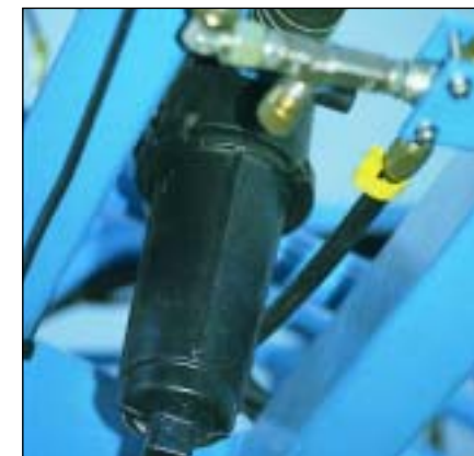
8 - In order to facilitate the maintenance of your sprayer, BERTHOUD recommends only one filter, 1/4 turn, at return to tank. As an option, if you wish, each section can receive an additional filter.
