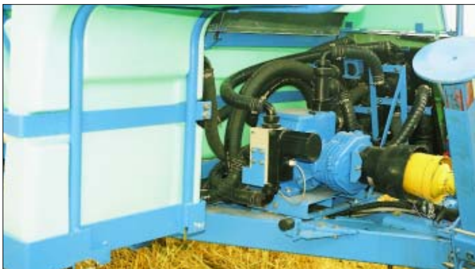
5 - Berlogic: Simplicity, ergonomics, reliability, for this start-up aid for your sprayer. A general chart groups together the operations that can be carried out: you just need position each valve on the number of the desired operation.
