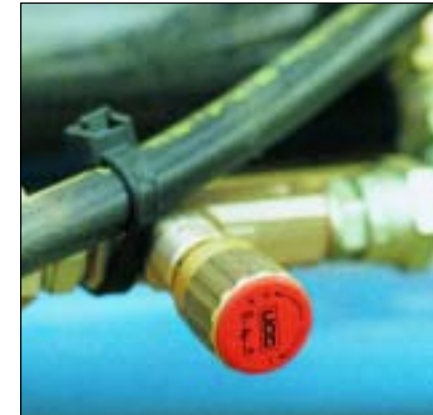
5 - On all the hydraulic functions, flow limiters enable the sprayer to be adapted easily to the oil flow and pressure of your tractor's hydraulic circuit.
