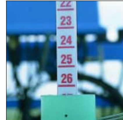
2 - Floating level gauge with direct read-out, visible from the tractor and from the filling point. Optionally, and notably with the Gestronic, the MAJORs can accommodate the Nivelec electronic gauge.
