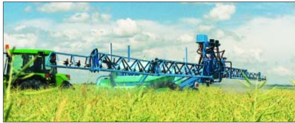
The MAJOR receives the "AXIALE" boom range of 24, 28 and 30 metres. (see leaflet AXIALE BOOM).
