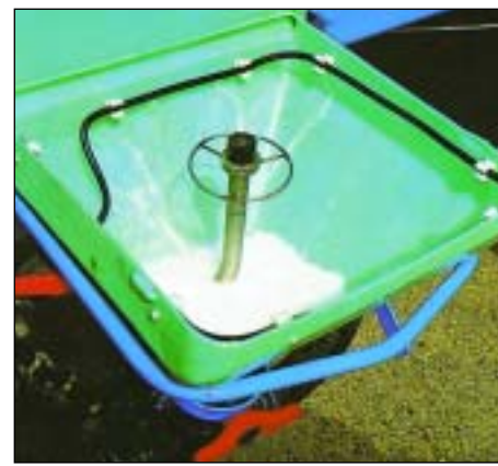
1 - Retractable chemical hopper, which is at man height at the time it is used and does not damage the vegetation during spraying; The hopper has a system which rinses chemical containers with a rinsing circuit. At the bottom a grill eliminates any blockage problems caused by caps and packaging.
