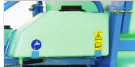
3 - Hand wash tank with a capacity of 18 litres, as per the European Community directives. It enables the operator to rinse himself in case of contamination by chemical products.
