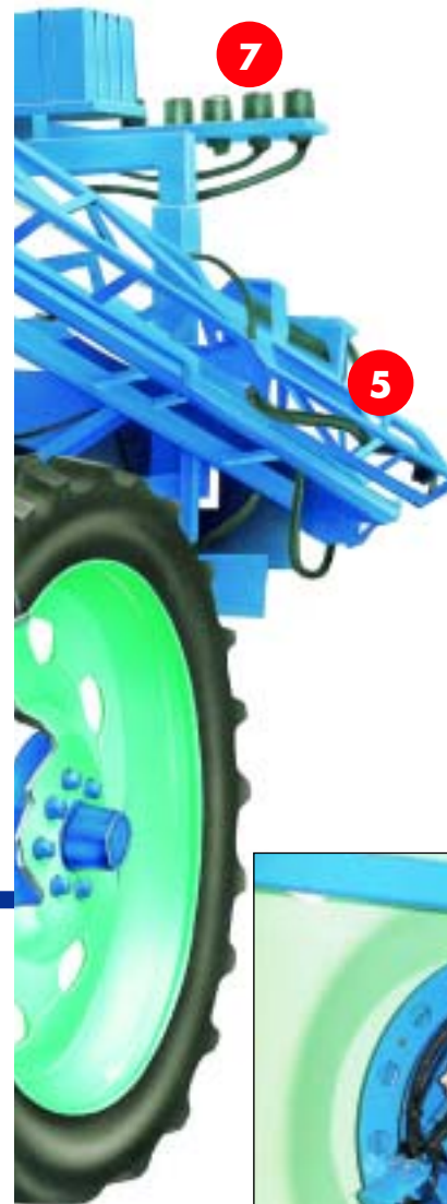
6 - As optional equipment, your sprayer can be equipped with a hydraulic braking system. Parking brake is standard. Input of information concerning ground speed is carried out on one of the wheels by a 16 impulse proximity sensor in order to obtain more accurate data.
