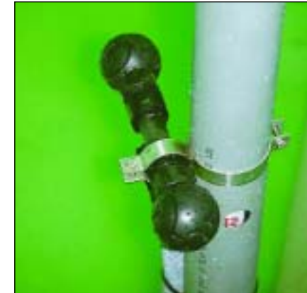
3 - In order to rinse out the tank after every application, a "Lav'ton" system is standard equipment on your sprayer. Do not forget to rinse out your tank between each spraying session.
