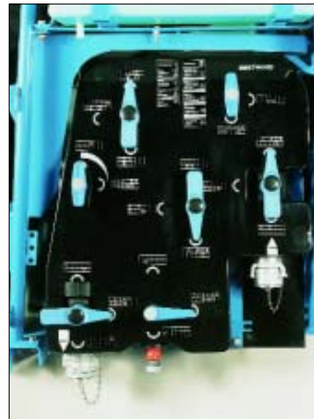
5 - Berlogic: Simplicity, ergonomics, reliability, for this start-up aid for your sprayer. A general chart groups together the operations that can be carried out: you just need position each valve on the number of the desired operation.
