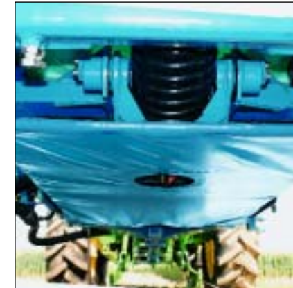
4 - As standard equipment, the MAJORs are supplied with a protective under-sheet so that, in periods of late spraying, the vegetation may slide easily under your sprayer.
