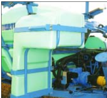
4 - A 280 litres rinse tank is standard equipment on the MAJOR. This capacity enables the circuit to be rinsed out immediately after spraying and before carrying out a thorough cleaning at the farm chemical store.
