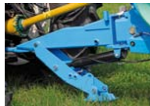
> Jackstand Choice of manual or hydraulic jackstand
