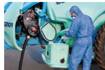
> Hopper Incorporating and rinsing chemical containers and spray circuit with clean water Large capacity (35L) with ergonomically-designed control lever
